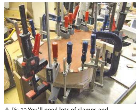
▲ Pic.20 You'll need lots of clamps and small cauls to spread the pressure on the curved sections
